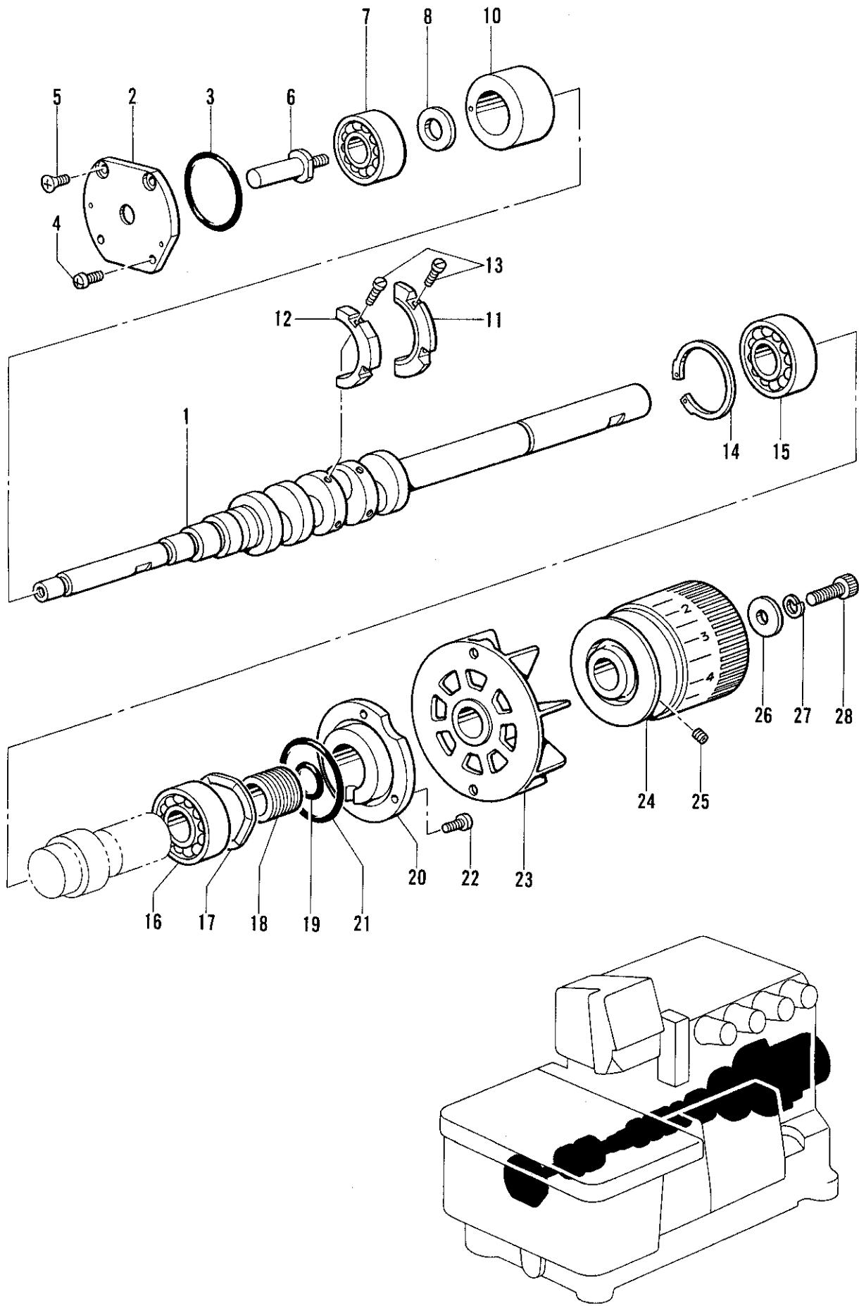
B. 駆動軸関係/Crank shaft mechanism/Kurbelwelle/
