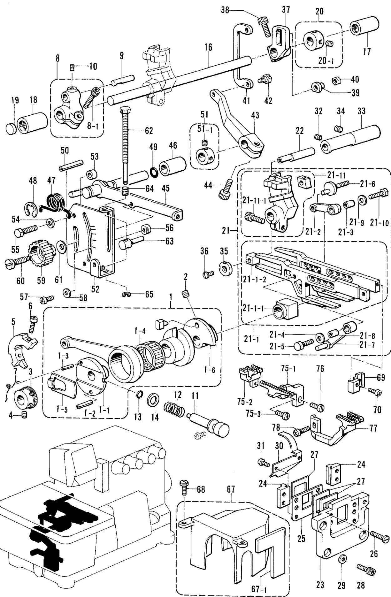
E. 送り関係/Feed mechanism/Transportvorrichtung/
