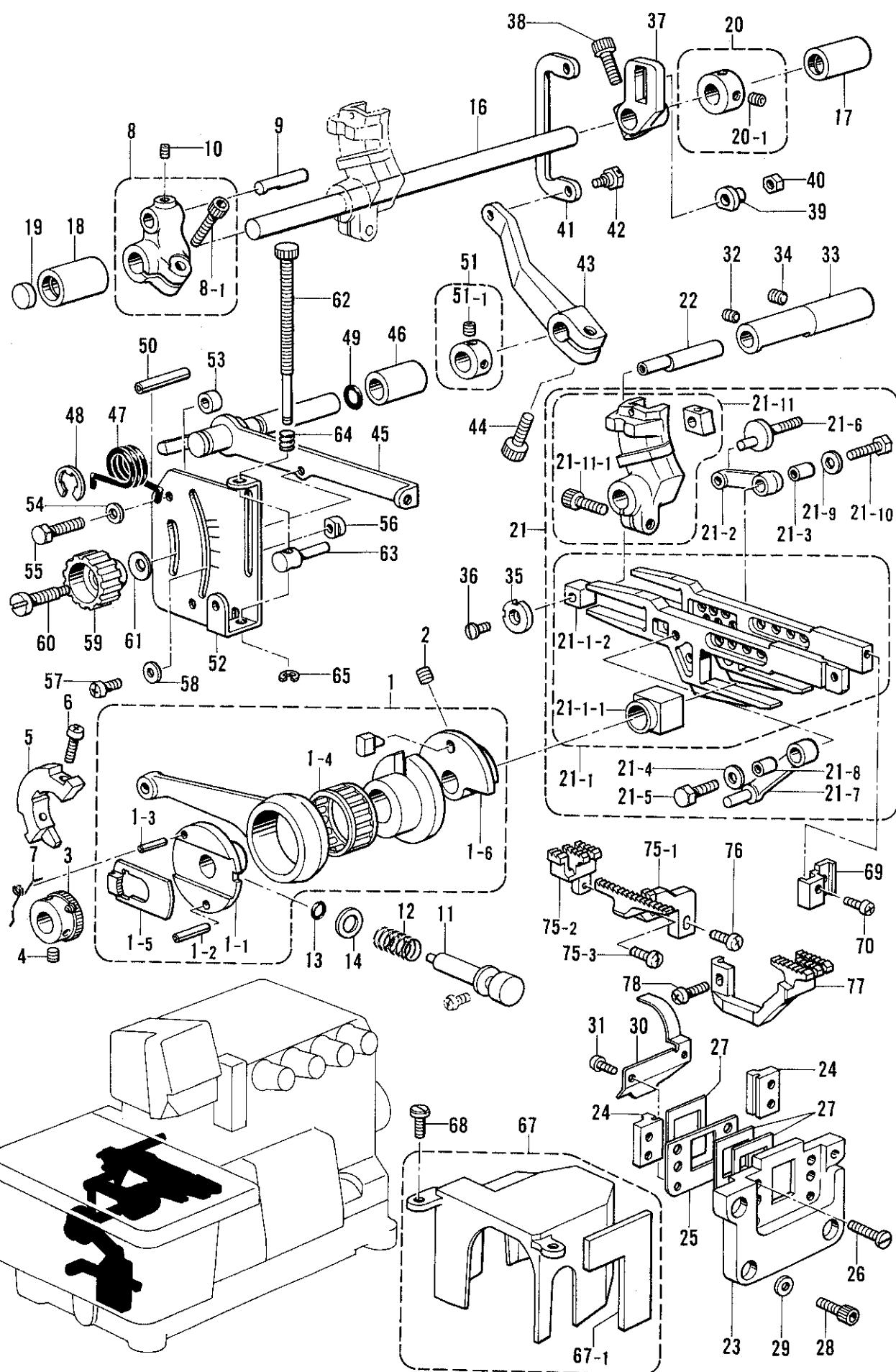
E. 送り関係/Feed mechanism/Transportvorrichtung/
